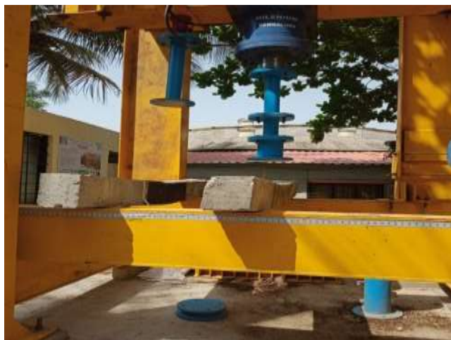
Fig.3 Testing of Beam under Loading Frame
